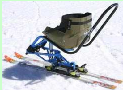
Abb 1.: The person accompanying is steering the „Dualski“ by means of the roll and push bar.
